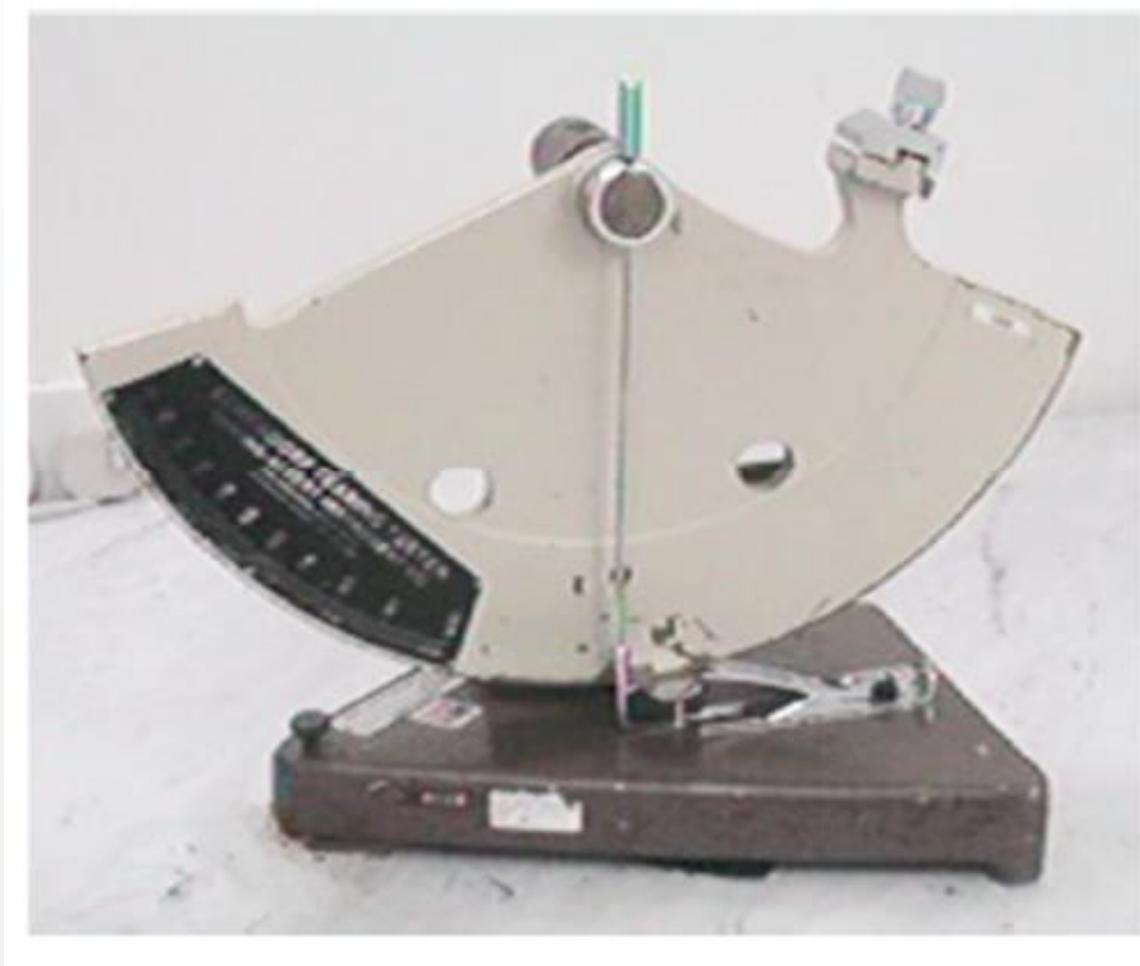
**Falling Pendulum Tester**
